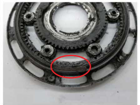
⑥ Wear and breakage of oil seal
