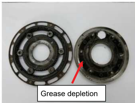
⑦ Depletion due to insufficient injection of grease
