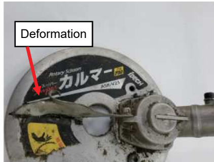
② Deformation of the stabilizer
