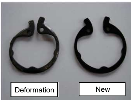
⑧ Deformation of the bottom disc fixing bracket
